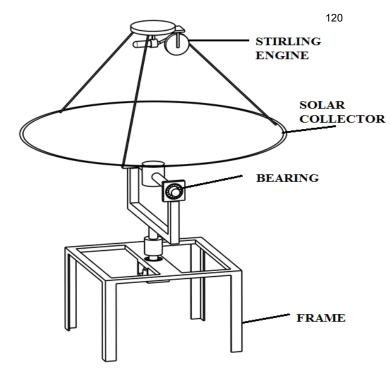
Fig 4.1: Construction of Setup for sterling engine.
